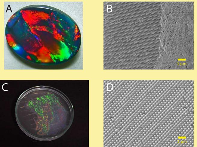
(A) Natural opal [downloaded from [static.opalauctions.com](http://static.opalauctions.com)]. (B) Self-assembled PS spheres of diameter 173 nm forming a synthetic opal (SEM micrograph). (C) Monolayer of self-assembled PS spheres of diameter 535 nm on water surface in a Petri dish. (D) Monolayer of self-assembled PS spheres of diameter 920 nm (SEM micrograph).
