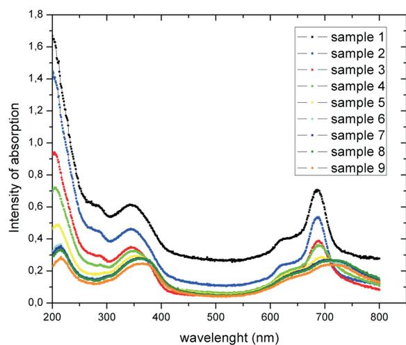
Figure 1: Absorption spectrum of mix Humic substances and phtalocyanines
