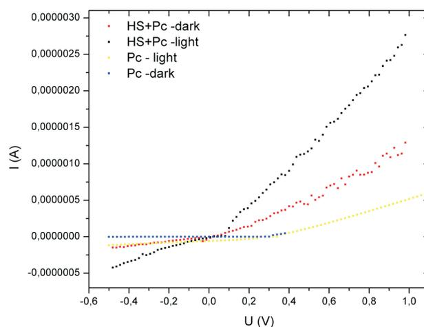
Figure 2: I-V characteristics of mix Humic substances with phtalocyanines and phtalocyanines.
