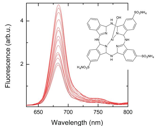
Figure 3: The fluorescence decrease with increasing concentration of quencher
