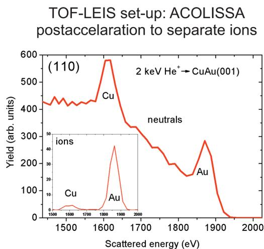
Fig. 1: Experimental spectrum of 2 keV He ions scattered from CuAu(001) - [110] azimuth. Au and Cu can be separated easily.
