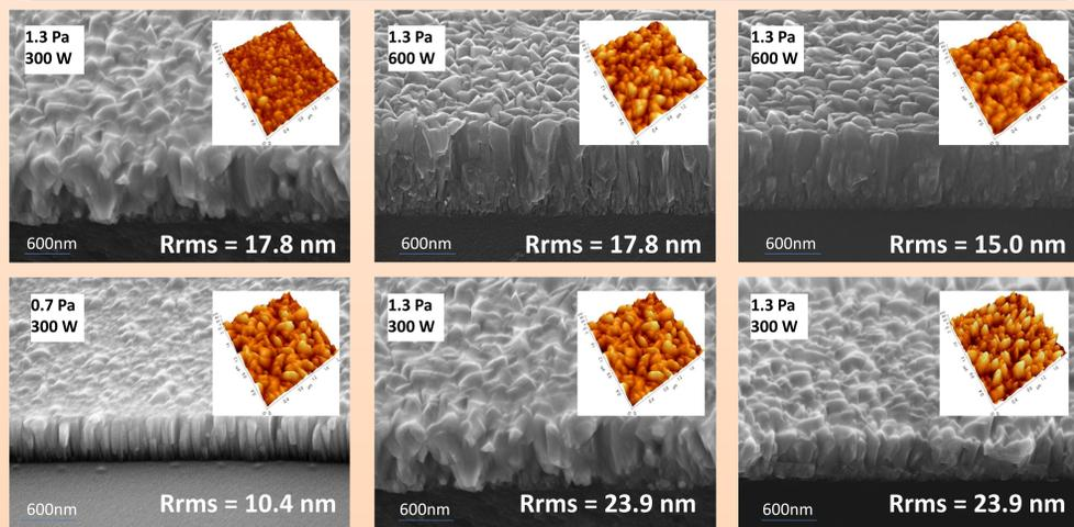
Comparison of SEM and AFM surface morphology of GZO thin films deposited by normal ( $S_n$ ) courses at different (1.3 Pa, 0.7 Pa) Ar pressure.
