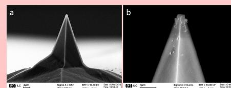
SEM image of many times measured standard tip
