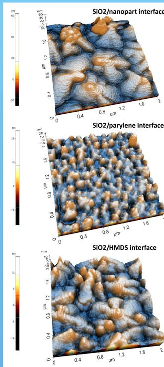
Influence of buffer layer on the parylene top layers resulted to very different structure of the molecular structure. Parylene is perspective material as a passivation material for its physical and insulating properties.
