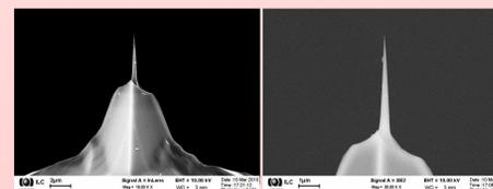
SEM image of new high resolution tip with high aspect ratio
