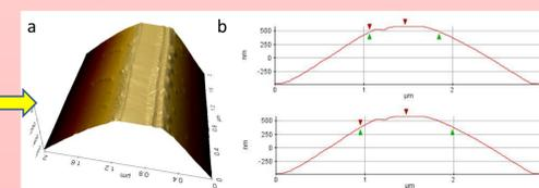
AFM image and line profiles of triangular step (2 x 2 μm)
