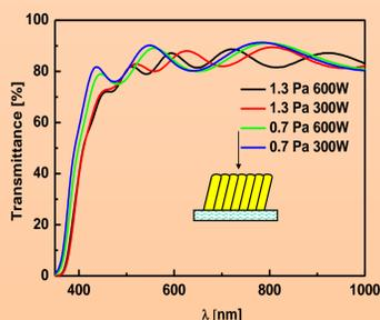
Spectrum of the specular transmittance in the range of 400 - 1000 nm of the normal ( $S_n$ ) and obliquely ( $S_o$ ) deposited films at different pressure and RF power.
