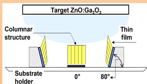
Oblique-angle sputtered GZO films by RF power of 600 W at room substrate temperature in Ar pressure 1.3 Pa showed the strong crystalline (002) texture, the lowest electrical resistivity  $3.4 \times 10^{-3} \Omega\text{cm}$ , the highest electron mobility  $10 \text{ cm}^2\text{Vs}^{-1}$ , high electron concentration  $1.8 \times 10^{20} \text{ cm}^{-3}$  and good optical transparency 88 %.
