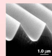
Fig. 4. SEM image of test grating - theoretical width of the step 100 nm below the top - 140 nm.
